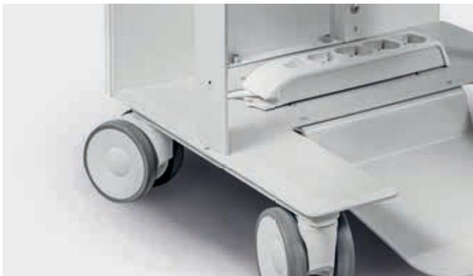
Smooth-running swivel castors with parking brake. Mounted on ball bearings with a load bearing capacity of 100 kg, thanks to their large diameter (100 mm) they are able to overcome obstacles such as: grouting, joining areas between different floors, small obstacles.
