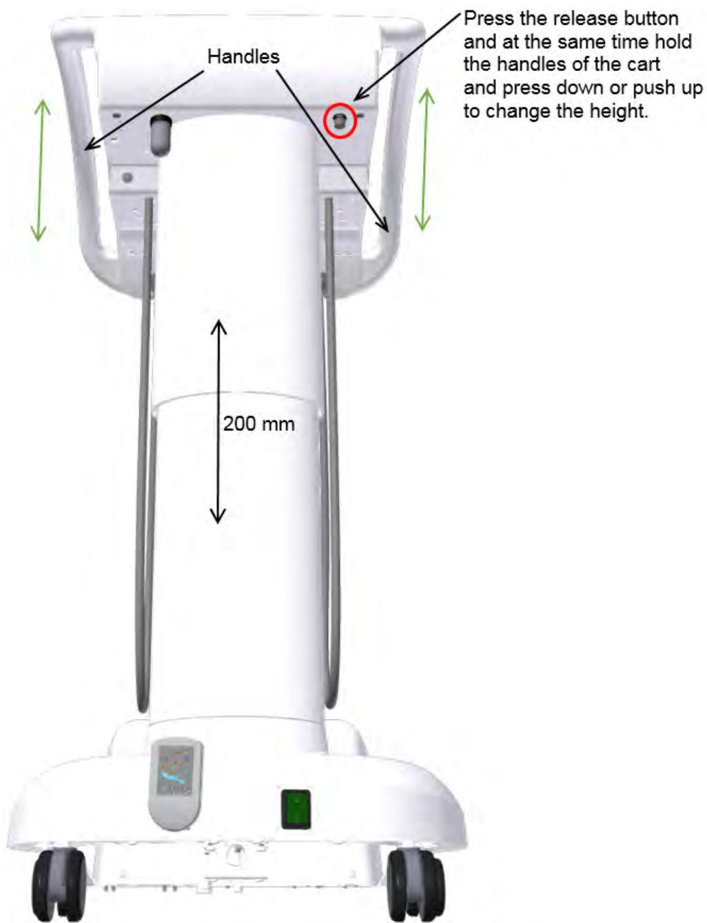
The working height of the control panel can be changed within the range of 200 mm. Grip the control panel (preferably while standing behind it) from the sides with both hands, while pressing (and holding) with a finger the button located on the bottom side of the panel, thus unblocking the mechanism of height adjustment. Re-position the panel gripped in the described way to the desired working height. Block the panel in the set height by releasing the mechanism button.
